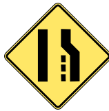
Lane Ends, Merge Left
